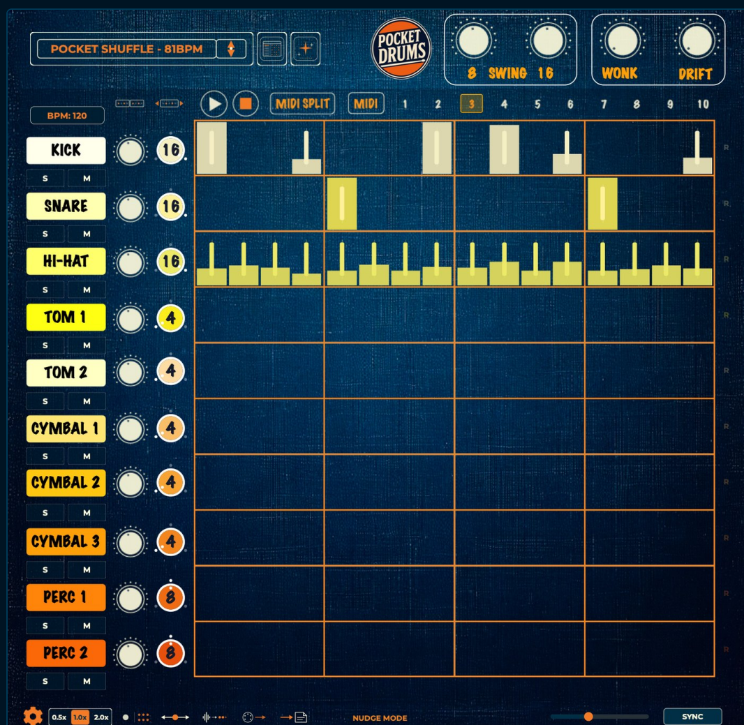
FIGURE 53.1 NUDGE MODE. Each handle sits at its step's total offset; the faint line is the grid position; R glyphs in the right margin reset a lane.
