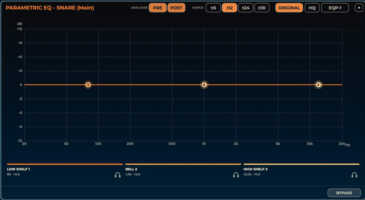
FIGURE 21.1 The Parametric EQ at its defaults: three legacy bands (low shelf 80 Hz, bell 1 kHz, high shelf 12 kHz), analyser PRE and POST on, ±12 dB range, ORIGINAL algorithm.
