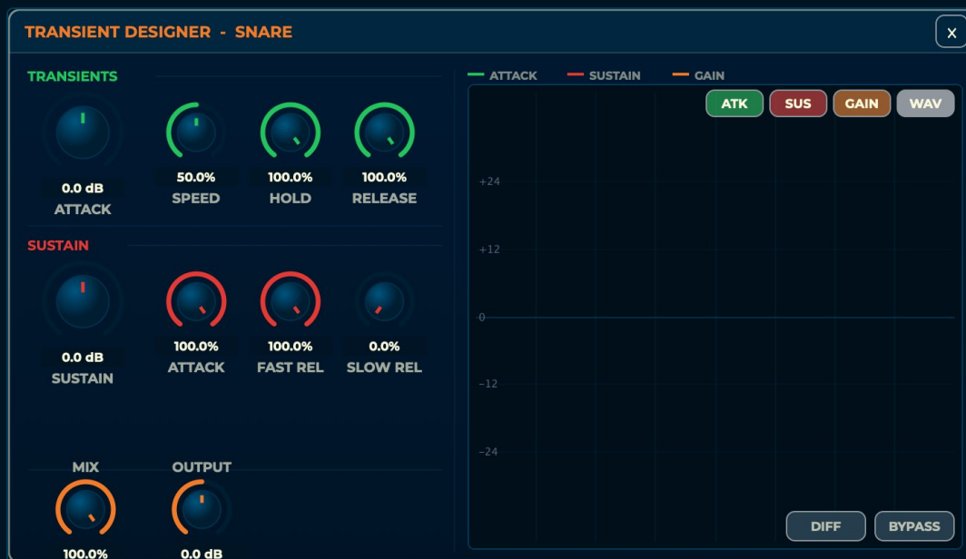
FIGURE 22.1 The Transient Designer at rest. The display shows one hit at a time with the live attack (green), sustain (red) and gain (orange) curves over the waveform once audio plays.
