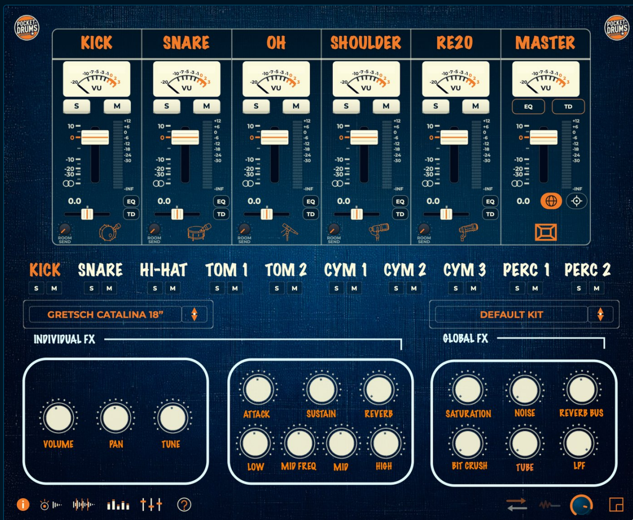
FIGURE 12.1 The console in the main view with a 5-mic KICK selected. It replaces the centre logo; everything below the headers is unchanged.
