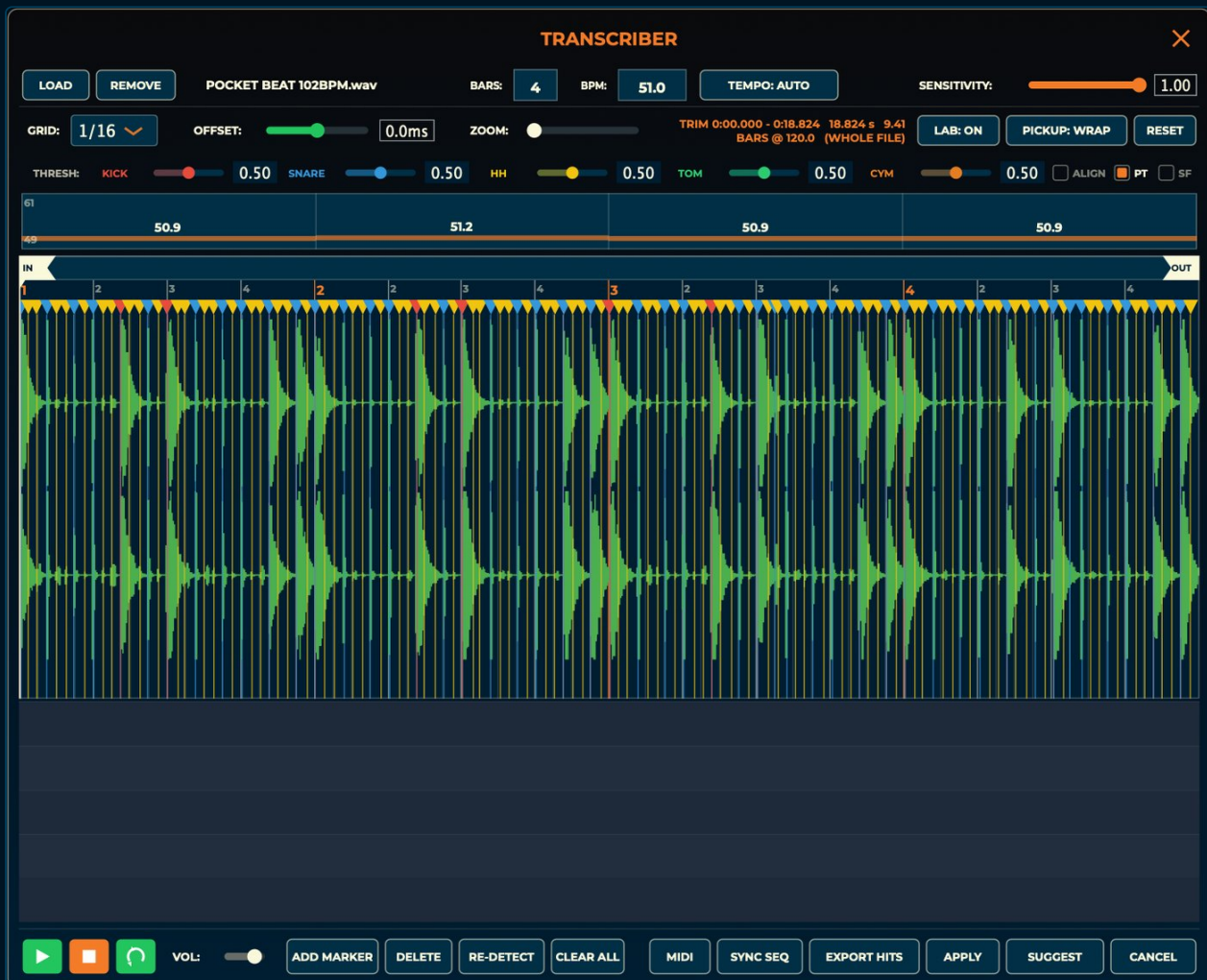
FIGURE 55.1 TRANSCRIBER with a loop loaded: settings rows, the five THRESH sliders, the tempo track, the waveform with class-coloured markers, the piano roll and the action row.
